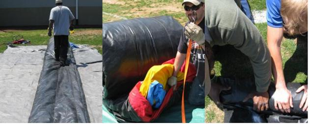
Step 2-6: Fold the Inflatable in 2-3 feet lengthwise and walk out air towards Ports (Blower tubes).
